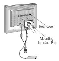
1 Align the Mounting Interface Pad with the holes in the Rear Cover and secure it with the four screws that came with the Arm-type Stand or Wall Mount Hanger.
